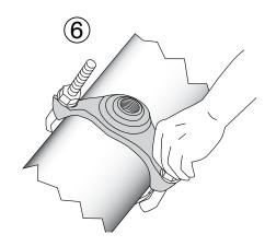
**Step 7** • Tighten all nuts evenly in 15-20 ft-lbs. increments. Use a wrench with at least a 12 inch handle.
