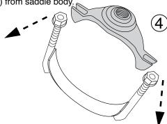
Step 5 • Position the saddle body on the pipe such that the outlet is in the correct location.
