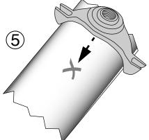
**Step 6** • Install strap(s) on saddle body, and tighten finger tight. Make sure the gasket has seated itself flat onto the pipe face.
