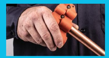
Step 2 Deburr the end of the pipe to remove any sharp edges.
