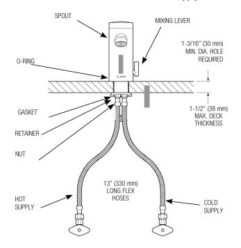
When the EAF faucet is installed on a sink that has three (3) hole punchings, a Trim Plate should be used. Trim Plates must be specified and ordered separately:
