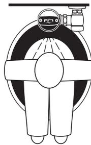
3. Once a user is detected, if the user leaves in 65 seconds or less, a reduced flush will automatically initiate. The circuit automatically resets and is ready for the next user.
