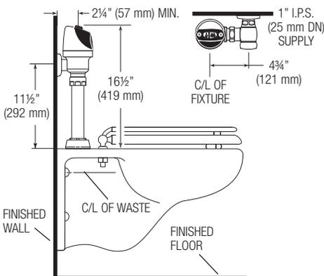
**When installing the Sloan ECOS® Electronic Dual Flush in a handicap stall:**
