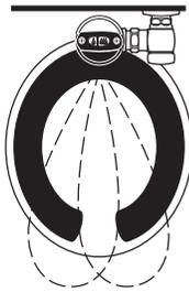
2. As the user enters the beam's effective range, 22" to 42" (559 mm to 1067 mm), the beam is reflected into the Scanner Window to activate the Output Circuit. Once activated, the Output Circuit continues in a "hold" mode for as long as the user remains within the effective range of the sensor. If the user stays longer than 65 seconds, a full flush will automatically initiate when the user leaves.
