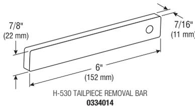
Sloan adjustable and ground joint tailpieces are assembled into the valve body using a pipe thread. Significant force is used to drive the tailpiece into the valve body. As such, removal of the old tailpiece may be difficult.
