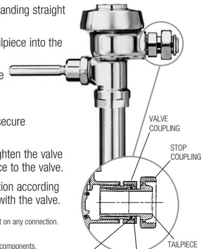
NOTE: DO NOT use pipe dope or thread sealant on any connection. Lubricate O-ring ONLY with water!
