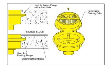
Most floor drain bodies are available with a flange for either anchoring the drain in the floor slab or for use as a flashing flange in upper floors and waterproofed areas. Many Smith drains are regularly furnished with a flanged body and a combination "top flashing collar" which can be used to clamp the waterproof membrane.
