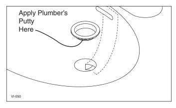
**Note:** When installing the sink ring and tail pipe, use plumber's putty sparingly and do not allow it to contact the plastic overflow assembly under the sink.
