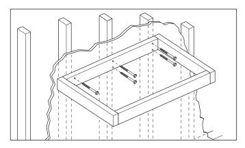
Trial fit the apron panel to the wall mount frame, checking for proper fit. Sand or trim panel, as needed. If installing apron panel to be ADA compliant, refer to the ADA Installation Requirements section for ADA requirements before installation.
