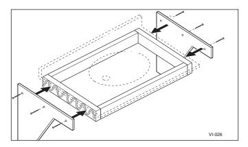
Note: The front apron strip must be cut to fit the overall width of the vanity.
