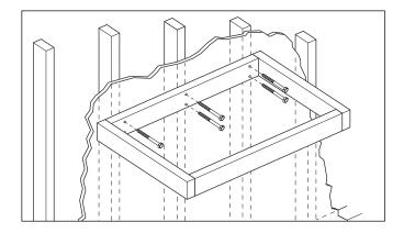
If the wall mount frame cannot be attached to at least two wall studs, cross blocking must be installed between the studs using 2 x 6 lumber.
