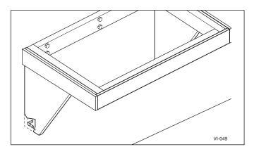
12. Clean underside of vanity sink with denatured alcohol. Remove all dust and let the surface dry completely.
