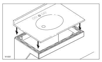
16. Wipe off any excess adhesive, and allow vanity top to set for 24 hours to ensure maximum adhesion. If the optional side splash panel is required, refer to Optional Side Splash Panel Installation section. 17. If desired, use a color-match silicone sealant (not included). Place a bead of sealant along the seam of the back splash panel and wall to create a moisture barrier.
