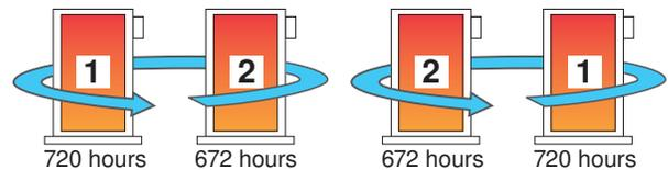
To reset the rotation sequence (without regard to historical running hours), toggle the Rotation DIP Switch Off for 3 seconds and on again. Note that the running hours (see Run Time) in the View menu also need to be reset if you want the rotation sequence and running hours display to be synchronized.
