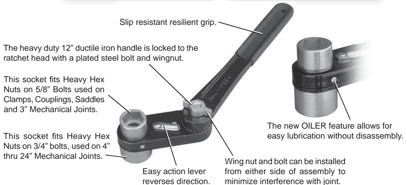
Adjustable head helps get to those hard-to-reach nuts and bolts!
