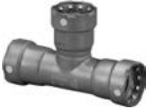
Viega MegaPressG is a carbon steel, cold press system designed for use in compressed air, fuel gas, and heating oil applications. Viega MegaPressG fittings are designed for use in piping systems utilizing ASTM A53, A106, A135 and A795
