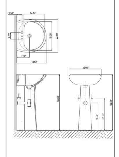
IMPORTANT: These dimensions are nominal and vary within the range of tolerances established by ASME standard A112.19.2
