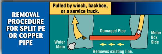
**REMOVAL PROCEDURE FOR SPLIT PE OR COPPER PIPE**
