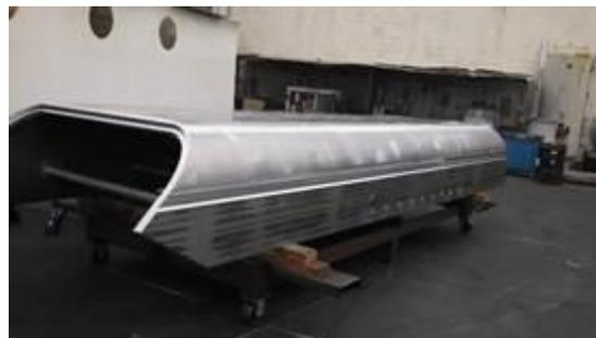
Finished formed and machined hull
