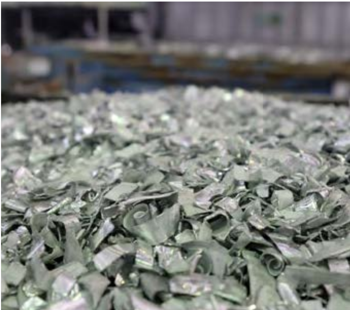
▲ Recycled input comes in all shapes—these are swarfs ready to be remelted
