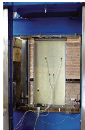
Compression load of 3 stringer panels: Comparison of bonding vs riveting
