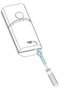
To open the battery cover, use a flathead screwdriver in the recessed slot as shown.
