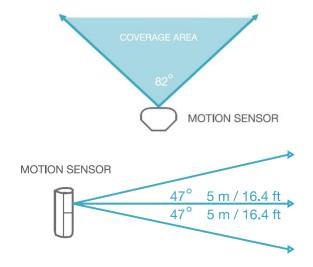
Orient the Motion Sensor for best use of its detection
