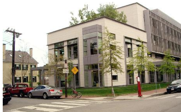
Sidewalks should be at least 6-8 feet wide, with wider sidewalks in areas of high-density and high-activity uses. Streetscape improvements should include repair of existing sidewalks, street trees, and street furniture like trash cans, pedestrian-oriented lighting, and seating.
