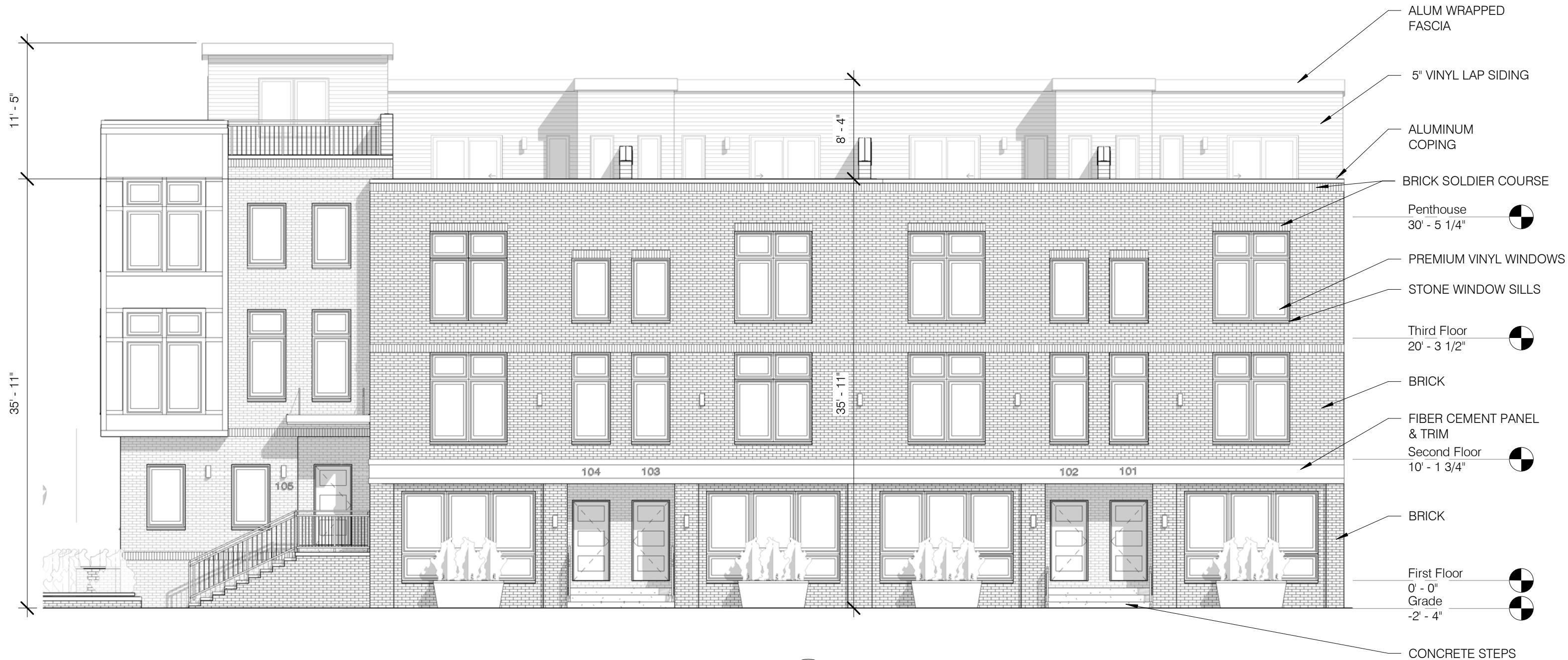
1 Units 1-5 South Elevation 1/8" = 1'-0"
