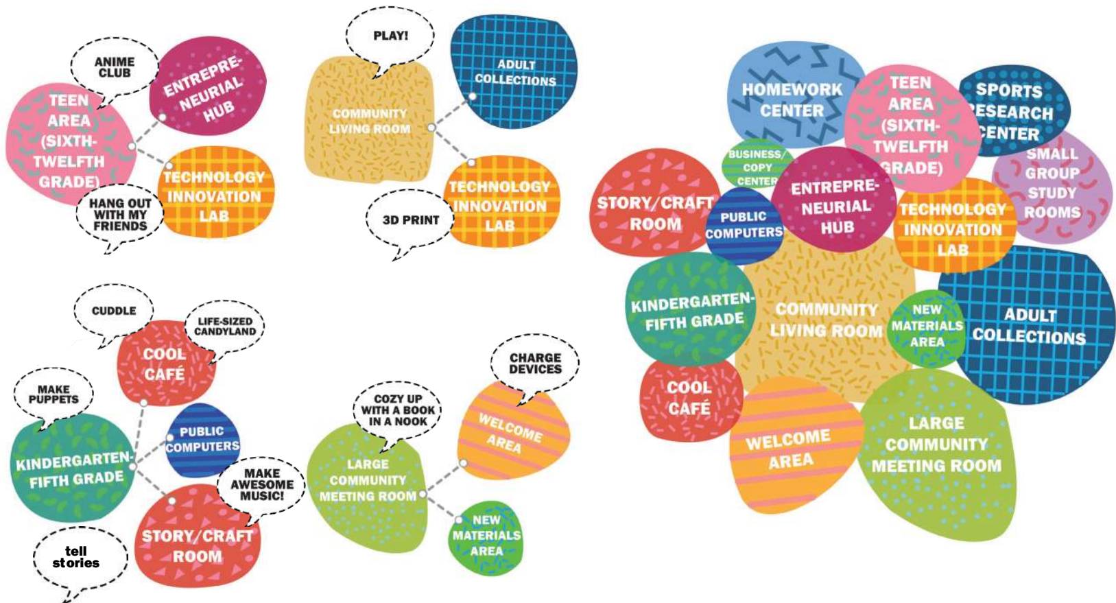
Examples of space adjacencies and activities and a concept diagram illustrating resulting from the activity.
