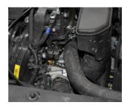
6. Reinstall all air snorkels ensuring any air flow sensors are properly installed and connected
