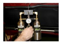
8. Turn Regulator clockwise and set pressure to 50-100 psi. Pressure should be adjusted based on engine displacement. For smaller 4 cylinder engines (2.0L and under) use 50 psi. For 6 cylinder and greater engines use up to 100 psi.
