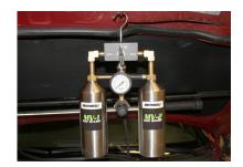
7. Hang Canister Assembly from the hood of the vehicle. Ensure Ball Valve is in OFF (Soak) position. Rotate Regulator fully counter-clockwise to ensure air supply is closed. Connect shop air. Connect Outlet Hose to the GDi Adapter.
