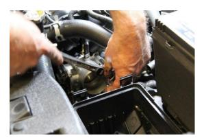
4. Unbolt Throttle Body from Intake and set bolts aside. NOTE: In some cases (Ford 1.6 & 2.0L) it is easier to remove the Intake and then Throttle Body.
