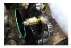
5. Place GDi Adapter in front of Throttle Body. Orientation of adapter should be with nozzle directing flow to intake valves. Secure GDi Adapter and Throttle Body with bolts provided.
