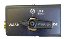
9. Start engine and set idle to 1700-2500 RPM. Turn Ball Valve to WASH and empty the contents of the WASH canister
