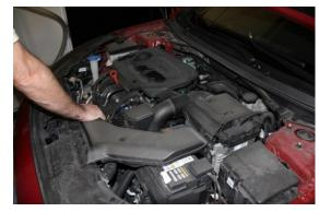
3. Remove Clean Air Snorkel (in some cases) and Snorkel from Air Filter to Throttle Body.
