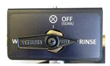
11. Turn ball valve to RINSE and empty the contents of the RINSE canister. Turn ball valve back to OFF (SOAK). Turn regulator fully counter clockwise, and disconnect shop air line from tool.
