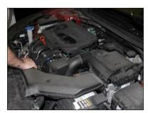
3. Remove Clean Air Snorkel (in some cases) and snorkel from air filter to throttle body.
