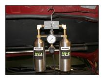
7. Hang canister assembly from the 8. Start engine and set idle between hood of the vehicle. Ensure ball valve is in **OFF** (Soak) position. Rotate regulator fully counterclockwise to ensure air supply is closed. Connect shop air. Connect outlet hose to the GDi adapter.
