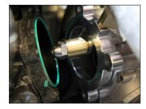
5. Place **GDi Adapter** in front of throttle body. Orientation of adapter should be with nozzle directing flow to intake valves. Secure GDi adapter and throttle body with bolts provided.
