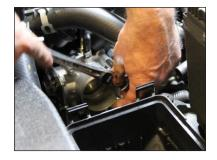
4. Unbolt throttle body from intake and set bolts aside. Note: In some cases (Ford 1.6 and 2.0L) it is easier to remove the
