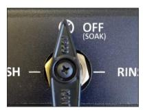
11. Turn Ball Valve to OFF (SOAK). Allow cleaning product to soak for **3-5 minutes** with engine running. Note: Snap throttle a few times to help clear any pooling of cleaner that may have accumulated. Repeat each time you select the OFF (SOAK) position.
