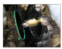
5. Place **GDi Adapter** in front of throttle body. Orientation of adapter should be with nozzle directing flow to intake valves. Secure GDi adapter and throttle body with bolts provided.
