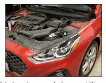
13. Let engine operate for an additional **3 minutes**. Turn engine off. Disconnect GDi Intake Tool and remove GDi adapter. Inspect intake for any pooling of products. If found, remove with shop towel. Failure to remove pooling may result in engine damage!! Install throttle body and air snorkels. Start engine and check that vehicle is operating properly. Perform a road test on vehicle (avoid aggressive driving maneuvers during road test).
