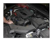
Remove Clean Air Snorkel (in some cases) and snorkel from air filter to throttle body.
