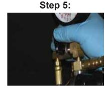
Ensure the vehicle is in park and start engine. Open gate valve slowly to allow GDi Induction System Cleaner to flow into Intake System.
