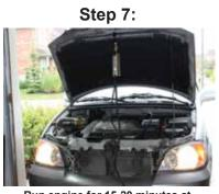
Run engine for 15-20 minutes at 3000 RPM. Monitor the fluid level through sight glass.
