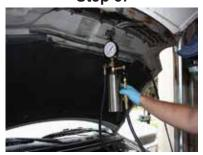
Open regulator to allow air into the bottle. Set regulator at 50-60 PSI.
