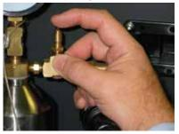
Press pin on schrader valve on regulator assembly to de-pressurize. Shut off engine, remove S-Tool. Reconnect the hose. The service is now complete.
