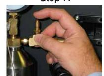
When the bottle is empty, close regulator, close valve on bottle and disconnect from shop air. Press pin on schrader valve on regulator assembly to de-pressurize.
