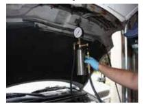
Open regulator to allow air into the bottle. Set regulator at 50-60 PSI.
