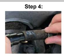
Insert into vacuum hose and secure with clamp.
