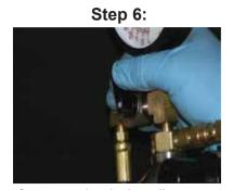
Open gate valve slowly to allow Valve Cleaner to flow into Intake System.
