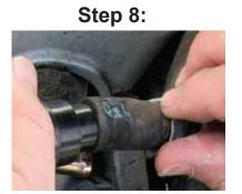
Shut off engine, remove S-Tool from vacuum line. Reconnect the vacuum hose. The service is now complete.
