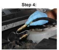
Attach S-Tool to air line from bottle. Place S-Tool into intake hose ensuring that the Mass Air flow sensor will not be sprayed.
