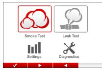
1. Select smoke test by pressing "select" button ( ) while smoke test icon is highlighted in red.
