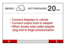
3. Follow on screen instructions and press the ( ) button to start pressurizing the system.
