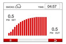
3. The screen displays the set pressure as well as the current output pressure. The test will automatically stop after 5 minutes.
