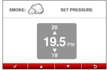
2. Set the test pressure by using the scroll buttons ( to adjust pressure. The test pressure should be the same or less than the operating pressure of the system being tested.
