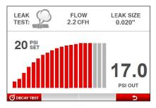
1. To perform a pressure decay test, begin a leak test. When the pressure has reached the set pressure, press the "Decay Test" button (Coccurrent).
