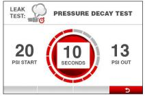
2. Follow The decay test will start the decay timer and show a live update on the screen of the output pressure. The time for the decay test can be changed in the options me.
