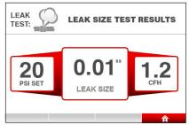
4. Results – When the output pressure stabilizes at the set pressure, the leak size results page will display the leak size and resulting flow rate from the test.
