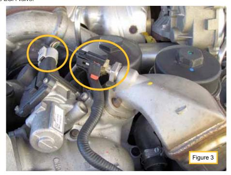
5. Install 069-3381 adapter (see figure 4) in place of above EGR temperature sensor.
