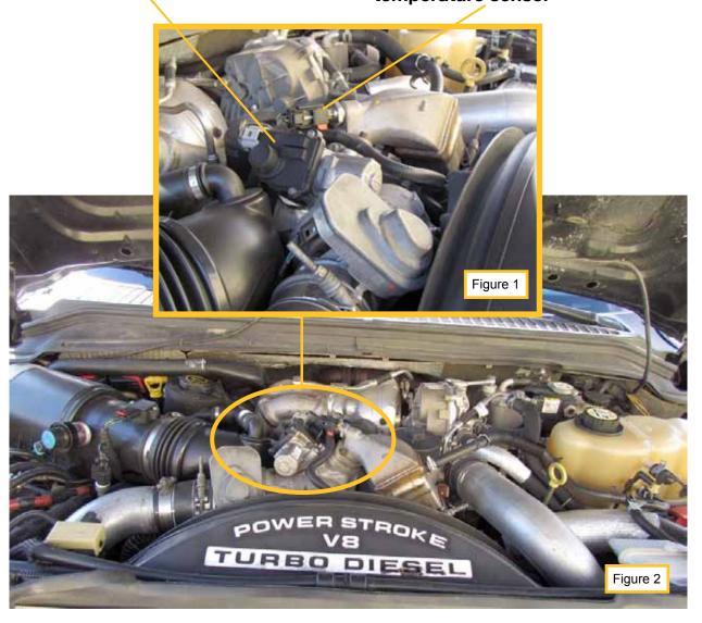
4. Remove EGR cooler temperature sensor (see figure 3). Disconnect EGR valve electrical connector to close the EGR valve.
