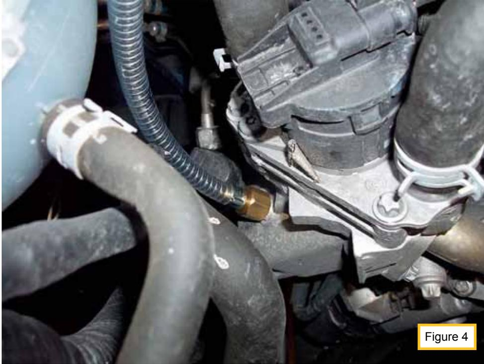
6. Attach aerator assembly to 069-3388. Ensure air valve and fluid valve are closed.
