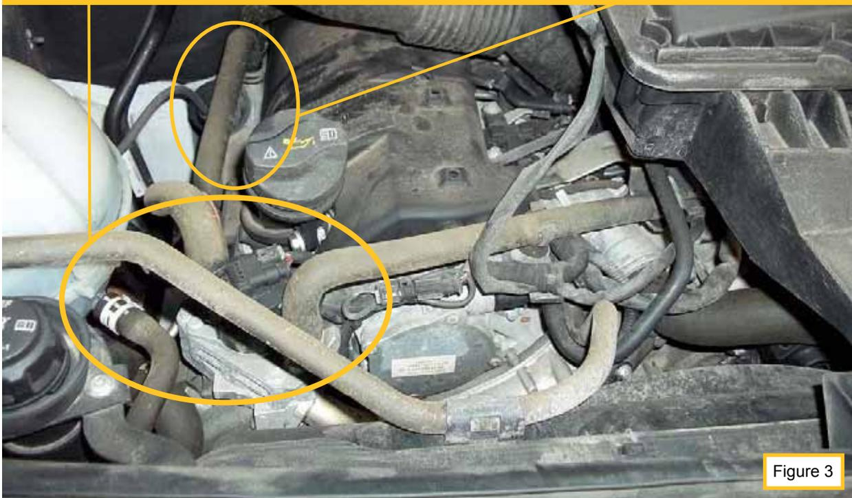
4. Remove EGR temperature sensor (see figure 1). Do not disconnect wire connector.
