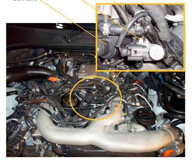
5. Remove EGR temperature sensor (see figure below) using a special 17mm socket. Do not disconnect wire connector.
