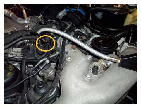
14. Using a scan tool, command the EGR valve and swirl flaps open.
