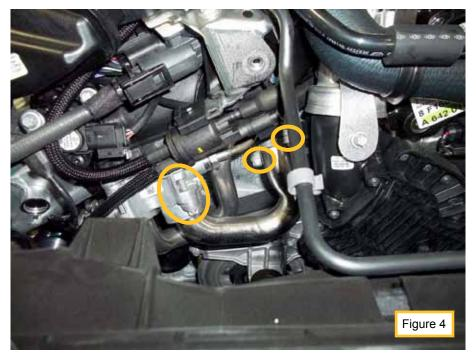
Quick Tip: Place the EGR cooler outlet pipe into a bucket/container and fill container with EGR fluid until submerged, this will aid in the dislodging of soot from the pipe while the EGR cleaning procedure is performed see step 21.
