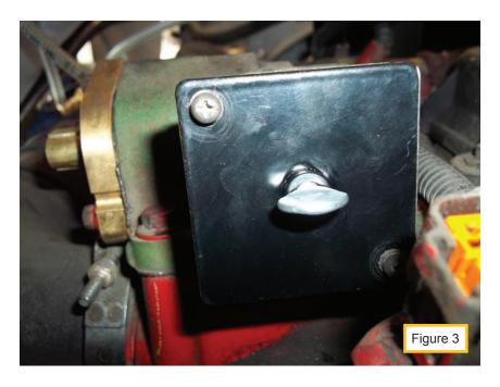
6. Install the EGR Intake Adapter (069-3576) using the two bolts 20mm (98821345) at the EGR valve and install the EGR Exhaust Adapter (069-3577) using the two nuts and bolts 60mm (98821345) supplied, on the EGR cooler outlet pipe. Tighten EGR cooler outlet pipe clamp (see Figure 4).
