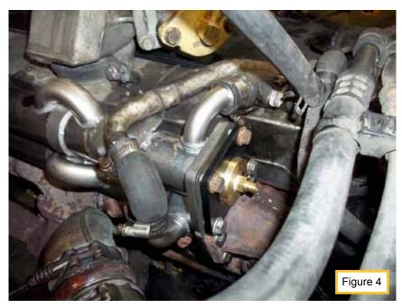
6. Attach EGR manifold 069-3399 to EGR adapters 069-3675. Attach EGR tool 500-0170 to 069-3399. Ensure air valve and fluid valve are closed – see EGR tool user guide.
