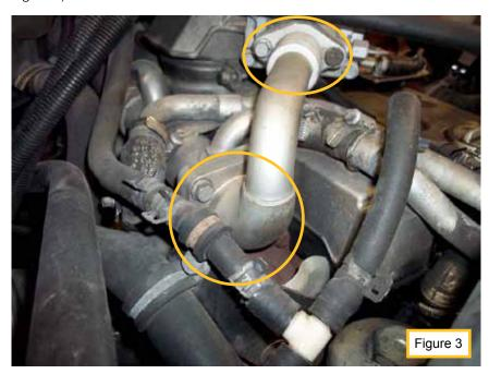
5. Remove the EGR cooler outlet pipe and set aside to be cleaned during service. Install EGR 069-3675 adapter' using the existing bolts (see figure 4).
