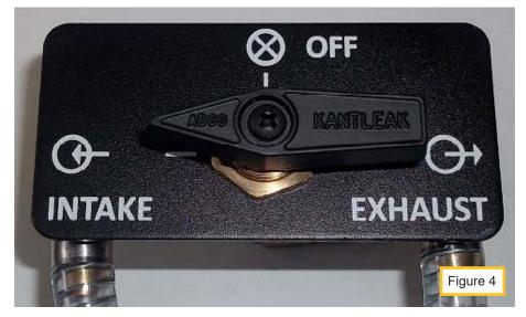
Quick Tip: To fully open EGR valve a hand vacuum pump the EGR Cleaning Tool can be used by connecting to the vacuum port on top of the EGR valve (see Figure 1 item "C"). NOTE: If at any time during the intake service you hear a diesel knock sound, turn the EGR Manifold to off for 2 minutes. After two minutes then turn the EGR Manifold to intake and continue service.
