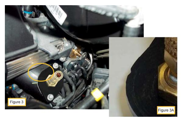
Quick Tip: Place the EGR cooler outlet pipe into a bucket/container and fill container with EGR fluid until submerged, this will aid in the dislodging of soot from the pipe while the EGR cleaning procedure is performed see step 14.
