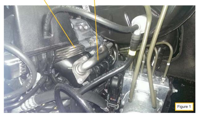
1. Remove EGR cooler outlet pipe by removing four bolts (see figure 2).
