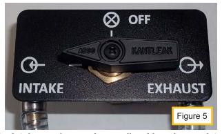
Note: If at any time during the intake service you hear a diesel knock sound, turn air and liquid valve on EGR tool closed for 2 minutes. After two minutes then turn air and liquid valve open and continue service.
