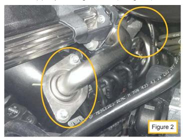
2. Install adapter 069-3530 in place of above EGR cooler outlet pipe (see figure 3) using the four bolts. The notch on intake adapter must be facing towards the engine for proper alignment and function (see figure 3A).
