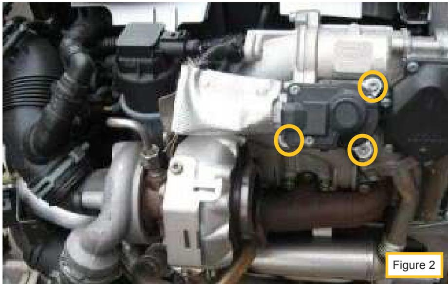
5. Remove EGR valve and set on top of engine with the electrical connector attached. Install 069-3565 in its place; install the 3 bolts hand tight.
