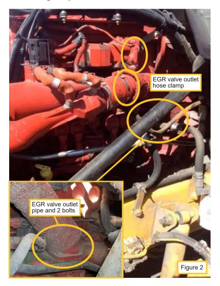
Quick Tip: Place the EGR valve outlet pipe into a bucket/container and pour EGR fluid into the outlet pipe, this will aid in the dislodging of soot from the pipe while the EGR cleaning procedure is performed.
