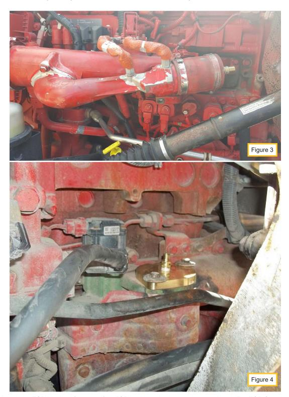
6. Attach the EGR Manifold (069-3399) to EGR intake and exhaust adapters. Attach The EGR Cleaning Tool (500-0170M) to the EGR Manifold. Ensure that the air valve and fluid valve are closed – see the EGR Cleaning Tool user guide.
