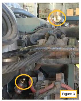
6. Attach the EGR Manifold (069-3399) to the EGR intake and Exhaust adapters. Attach the EGR Cleaning Tool (500-0170) to the EGR Manifold. Ensure that the air valve and fluid valve are closed – see the EGR Cleaning Tool user guide.
