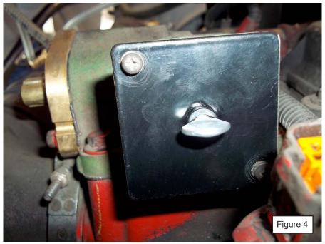
Note: For easier installation of the EGR manual valve opener, it is best to remove EGR valve assembly first (4 bolts). Install EGR Manual Opener and then reinstall EGR valve assembly.
