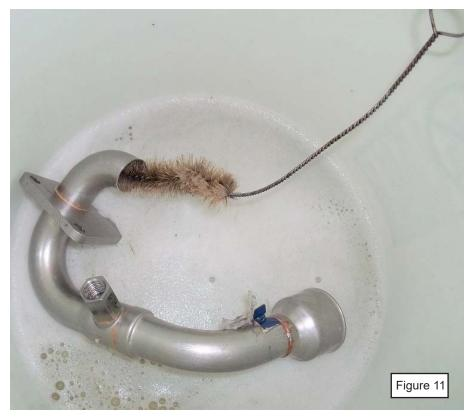
20. Remove EGR Adapters and reassemble vehicle components in the reverse order of removal. Wipe off EGR temperature sensor using the EGR cleaning fluid before installing.
