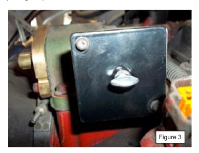
6. Install the EGR Intake Adapter (EEDF400-576) using the two 20mm bolts (98821336) at the EGR valve and install the EGR Exhaust Adapter (EEDF400-577) using the two nuts and 60mm bolts supplied, on the EGR cooler outlet pipe. Tighten EGR cooler outlet pipe clamp (see Figure 4).
