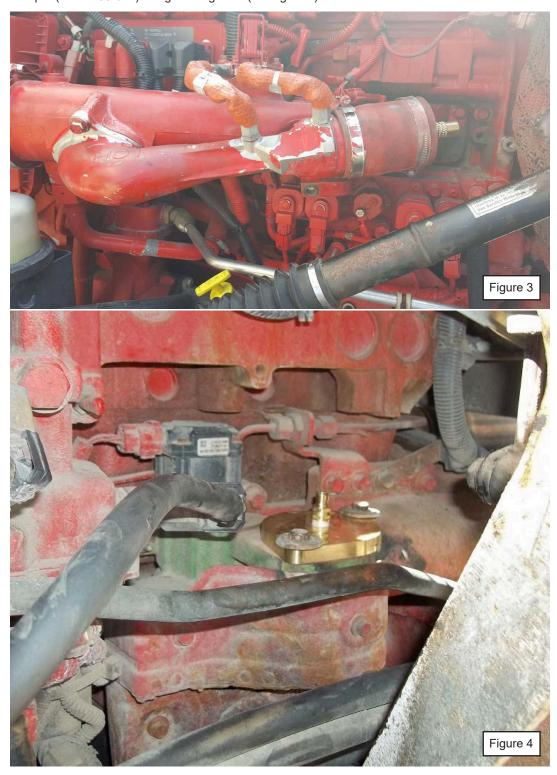
6. Attach EGR manifold (EEDF400M) to EGR intake and exhaust adapters. Attach EGR tool (EEDF400) to EGR Manifold. Ensure air valve and fluid valve are closed – see EGR tool user guide.
