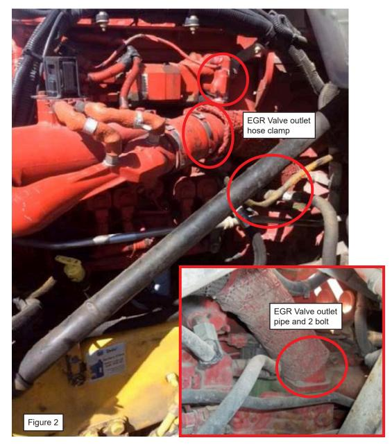
Quick Tip: Place the EGR valve outlet pipe into a bucket/container and pour EGR fluid into the outlet pipe, this will aid in the dislodging of soot from the pipe while the EGR cleaning procedure is performed see step 14.
