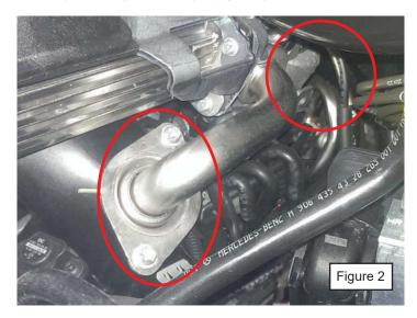
5. Install EGR Intake (EEDF400-531) and Exhaust (EEDF400-532) Adapters in place of above EGR cooler outlet pipe (see figure 3) using the four bolts. The notch on intake adapter must be facing towards the engine for proper alignment and function (see figure 3A).
