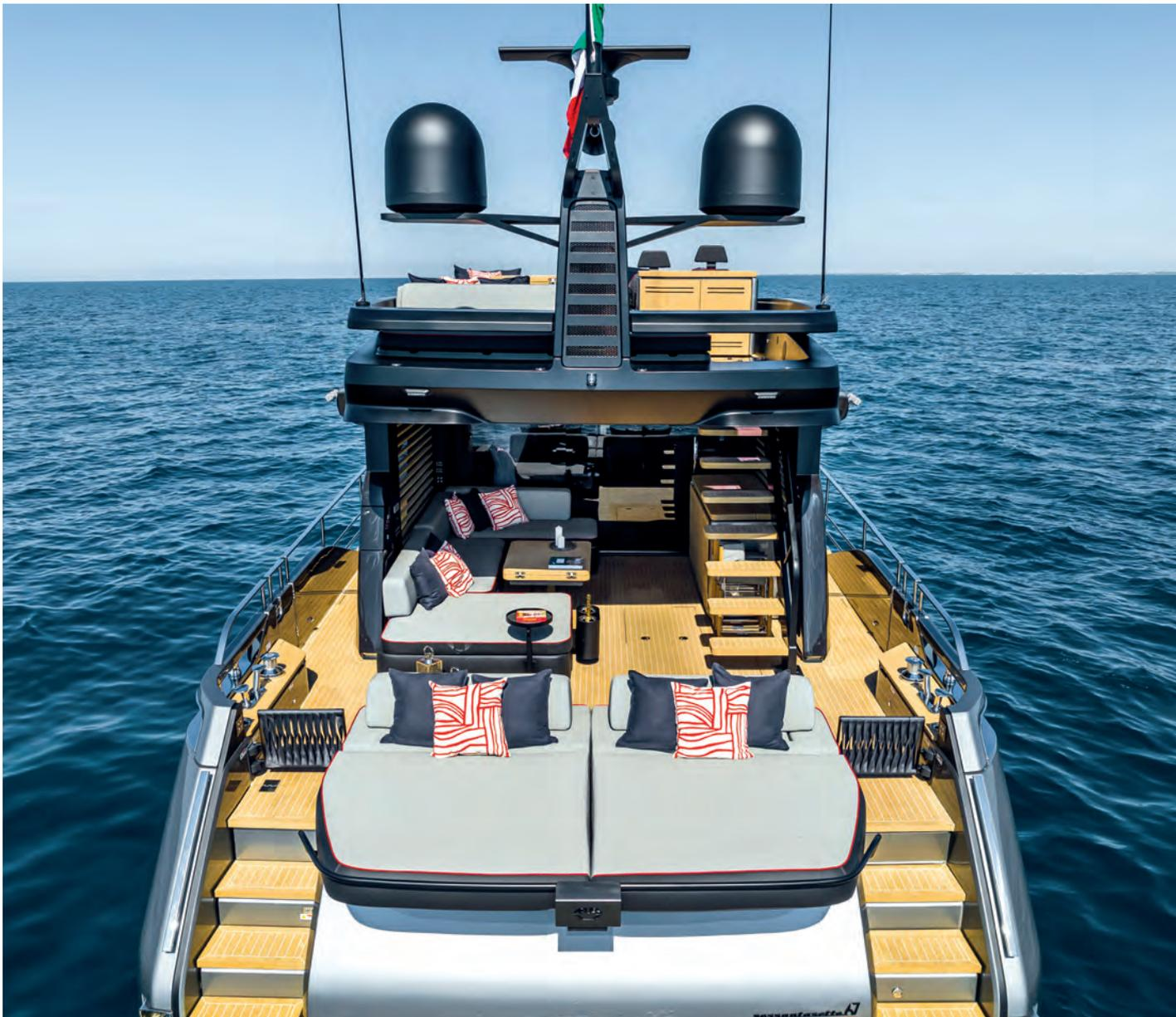
An evolution of the Cranchi Sessantasette 67 Fly, the new Corsa, this too designed by Christian Grande, is 20.80 metres long, 5.45 metres wide and has a displacement of 41 tonnes. The engine room houses two Volvo Penta D13 1,000 hp engines with IPS propulsion. The hull was designed by Aldo Cranchi.
