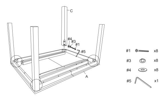
Step 2. Attach support bars (part B) to table top (part A) using bolts (part #2), spring washers (part #3), flat washers (part #4) and wrench (part #5).
