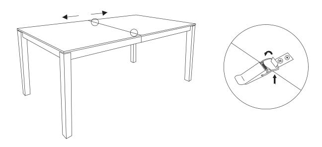
Step 4. Place table leaf (part D) in position and push table top (part A) from both ends to close.
