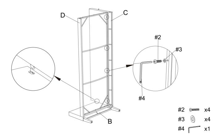
Step 3. Attach right arm panel (part A) to seat panel (part D) and back panel (part C) using short bolt (part #1), long bolts (part #2), flat washers (part #3) and allen wrench (part #4).
