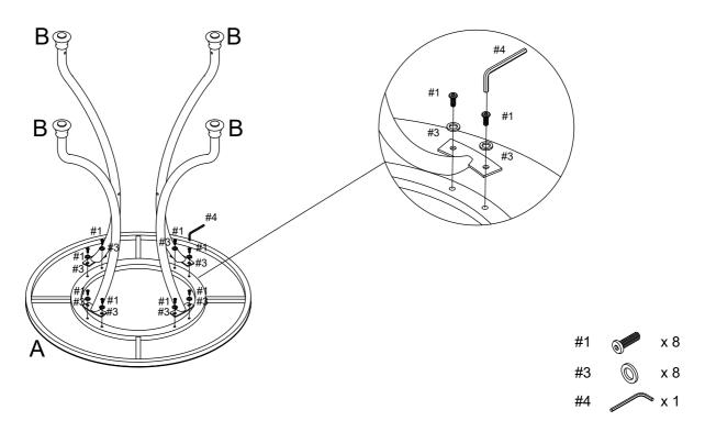
Step 2. Attach circle frame (part C) to legs (part B) using long bolts (part #2), washers (part #3) and allen wrench (part #4).
