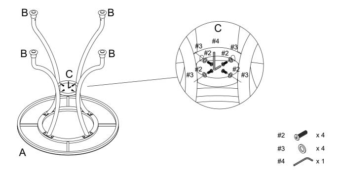
Step 3. Attach bottom frame (part D) to legs (part B) using bolts (part #1), washers (part #3) and allen wrench (part #4).
