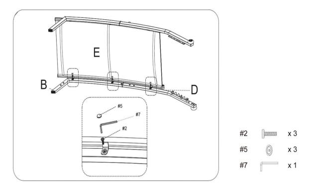
Step 5. Attach support tube (part G) to seat (part E) using medium bolts (part #2), plastic caps (part #5) and allen wrench (part #7).
