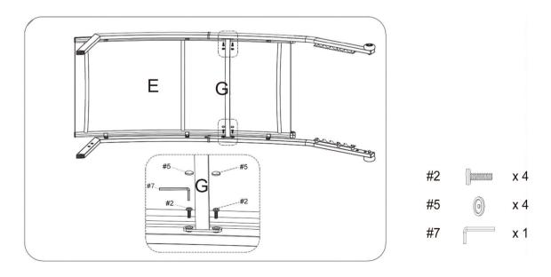
Step 6. Attach middle pole (part H) to legs (parts A & B) using medium bolts (part #2), plastic caps (part #5) and allen wrench (part #7).
