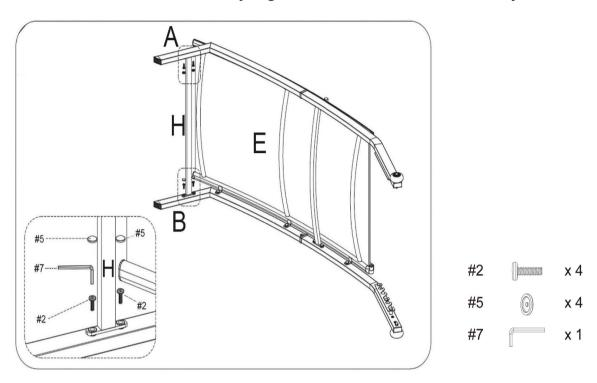
Step 7. Attach middle pole (part H) to back legs (parts C & D) using medium bolts (part #2), plastic caps (part #5) and allen wrench (part #7).
