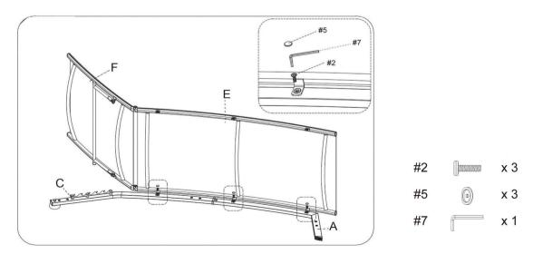
Step 4. Attach seat (part E) to assembled unit (parts B & D) using medium bolts (part #2), plastic caps (part #5) and allen wrench (part #7).
