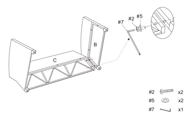
Step 3.Attach center seat panel (part #D) to assembled parts (part #A,C & B) using short bolts (part #1), long bolts (part #3), washers (part #5), nuts (part #4), wrench (part #6) and allen key (part #7).
