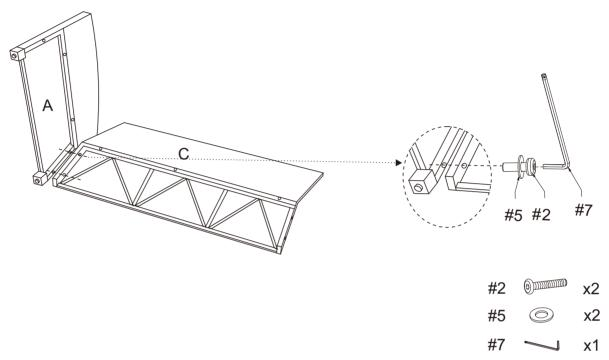
Step 2. Attach right arm panel (part #B) to back panel (part #C) using the medium bolts (part #2), washers (part #5) & allen key (part #7).
