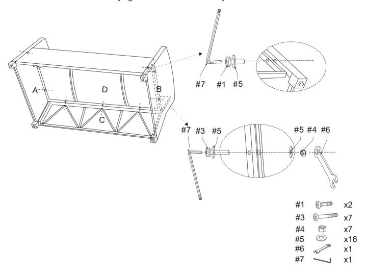
Step 4.Attach center leg (part #E) to seat panel (part #D) using short bolts (part #1), washers (part #5) and allen key (part #7).
