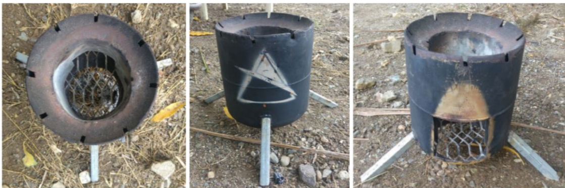
Figure 1. Photo of prototype Rocket Stove, view from top and sides
