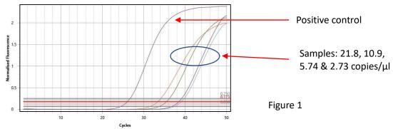
We were able to consistently pick up samples with a median of 2.73 copies/ $\mu$ l (the product from Vircel is delivered with a range of of virus per ml).
