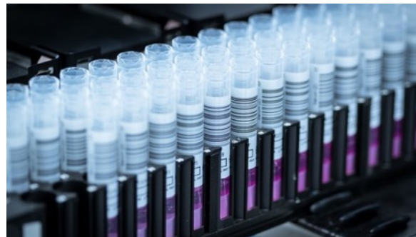
Hand fed onto Tecan liquid dispenser Caps have to be taken off, swab removed and barcodes need to be read
