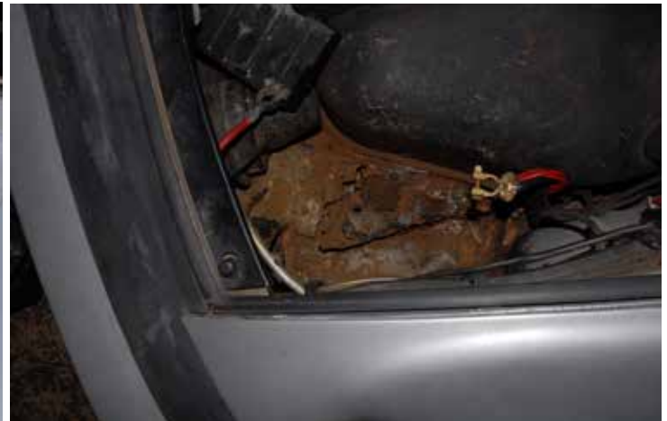
Why you should remove the battery when doing a PPI, especially on an older 911.
