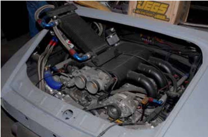
A souped-up Subaru boxer motor jammed into an older 911 chassis. At 450 hp, Sean thinks the engine is more than the chassis and the customer can handle.
